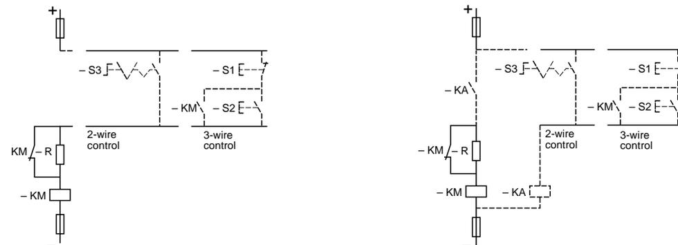
It is essential to check that the control circuit contacts have ratings compatible with the voltage and power consumption of the operating coil of the contactor. If not, an intermediate "KA" relay must be fitted and wired as shown.
